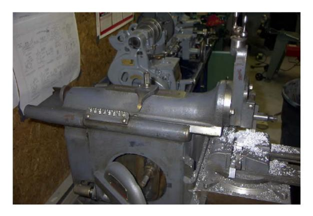
The ram can also be positioned to move the stroke in or out in relation to the table. This particular shaper had an indicator plate on the shaper housing with a pointer on the ram to show the stroke. To adjust this the nut holding the pointer is loosened and the knob at the rear is used to adjust the position of the ram.
