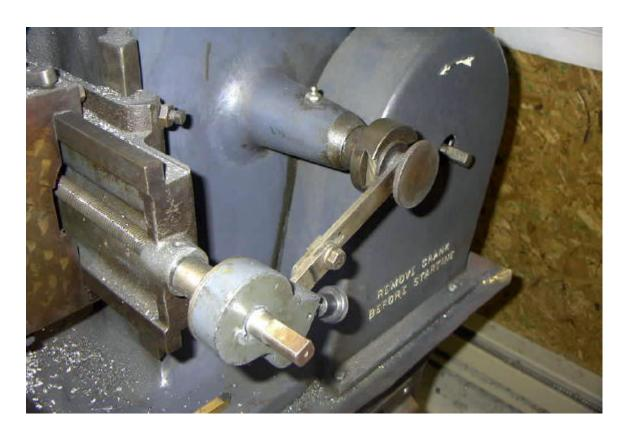
Make sure that the two-piece feed linkage remains straight. Initially mine was flexing like an elbow and only allowing for a partial advance of the table on each stroke because of the lost motion. When I adjusted it to the correct length and tightened it down the feed improved immediately.
