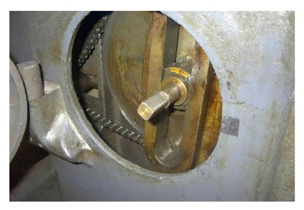
The photo above shows the chain drive and the stroke adjustment. By loosening the central nut and moving the assembly the length of the stroke is changed. Keeping it in towards the center of the yoke gives you a short,
